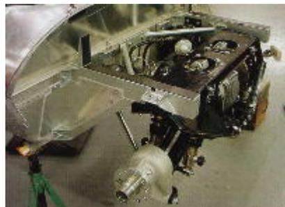
While the Lynx XKSS re-creations gain sophistication in ride and handling by using the E-Type independent rear suspension, their body construction is very much similar to the original's. The XKSS was the road-going version of a Le Mans winning D-Type racer, so naturally the entire body is made from lightweight aluminium. The front and rear body sections are welded or riveted together then attached to the central steel monocoque.
