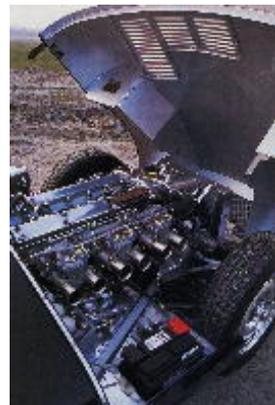
Continuing the theme of traditional tuning, big valves with a three-angle grind were installed, and the cylinder heads ported, polished and matched to the intake and exhaust manifolds. High-lift cams with a 0.45 thou lift and 282° duration were installed, along with stronger valve springs. It's a thorough job.
