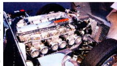
The compression ratio is a relatively modest 8.785:1 to cope with possible poor fuel quality. With gas-flowed heads and those triple Weber 45 DCOEs, the big XK motor produces 320bhp at 5,400rpm with 350lb ft of torque at 3,800rpm.
