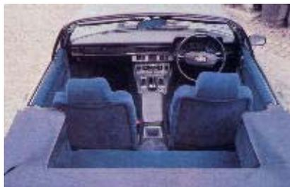
**SUPERB WORKMANSHIP** - Lynx have taken the opportunity to operate the rear quarter windows electrically (they rotate, rather than rise or fall), providing an instant pillarless coupe or convertible at the touch of the respective switches. The standard of workmanship and design is superb — just about the only aspect of the XJS Spyder that can be criticised from an aesthetic viewpoint is the
