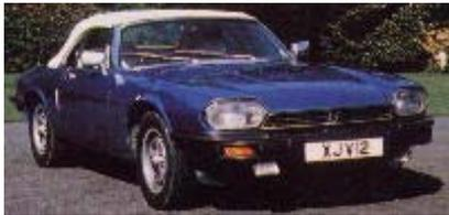
Certainly, the body finish is good, and the hood mechanism itself works very well. To lower the hood the procedure is as follows: first detach the two chunky windscreen top bar clips, then lower all the windows, especially the rear ones. The switch for the power mechanism is in the central cubby, and once the hood is lowered there is a cover for it attached by press- studs. Again, on the test car, this was of the dreaded PVC and had shrunk somewhat; the mohair ones should be easier to operate.
