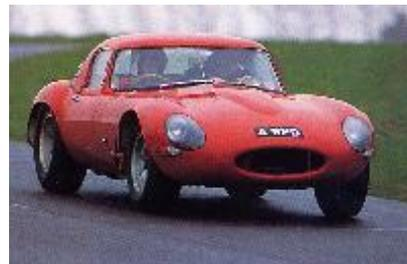
At the end of 1961, the Coombs car, BUY 1, was re-registered 4 WPD and, during the winter, it received an aluminium bonnet and hardtop and a new monocoque in lighter gauge steel. It was also fitted with a D-type wide-angle cylinder head with triple Weber 45 DCOE carburettors, larger brake discs, a brake servo, stiffer suspension and a 26-gallon fuel tank. Basically a works development car, 4 WPD was still not yet a Lightweight.
