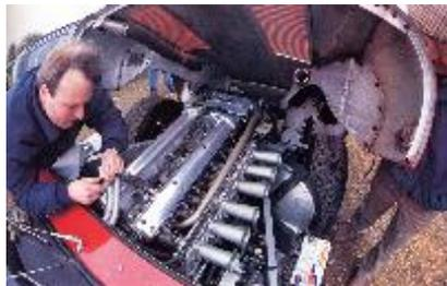
Most Lightweights produced 300-310bhp (a Ferrari 250GTO had 300bhp) but, by the end of 1963 development on 4 WPD had raised power to 344bhp thanks to the use of a sliding plate throttle and tuned exhaust. The only other Lightweight to receive these mods was the Lindner/Nocker car which ran at Le Mans in 1964.
