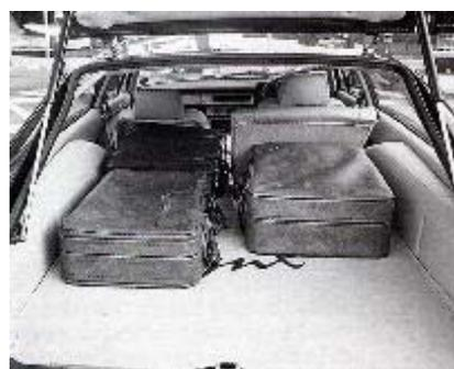
The beautifully crafted tailgate swings upward on a pair of gas struts to reveal a useful-sized opening which extends down to rear bumper level, thus facilitating easy loading and unloading of awkward-shaped objects. A lockable compartment in the left rear wing provides a useful amount of secure storage space, while a similar one on the right side houses the electronics, battery rear screen washer bottle and retracting aerial mechanism. The spare wheel is slung under the loadfloor.
