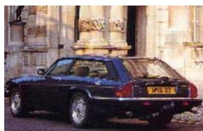
The changes add 60kg (132lbs) to the weight of a standard XJS, but this is balanced off by the fact that the improved aerodynamics of the longer roofline make for a more efficient shape which, all else being equal, endows the Eventer with a 2-3mph higher top speed. The vehicle's centre of gravity is also moved rearwards by 3 in. which has a slight beneficial effect on handling.
