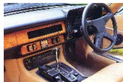
As part of the £16,000 (plus VAT) price tag for the conversion, Lynx includes a certain amount of mechanical refurbishment and refitting of the original vehicle. The interior, for instance, remains Jaguar through and through, but is retrimmed to original vehicle standards using high quality carpet, English woolcloth for the headlining and Connolly hide for the new rear seats, which also feature a 50-50 split folding backseat.
