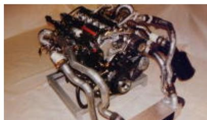
and oil-cooled, protecting the bearings in the best way possible. All that remains of the original 3.8-litre engine is the block which, most importantly, has had added oil cooling jet pipes which go through the block and spray a mist of oil on to the piston crown bottoms. This neat little modification helps reduce the heat build-up and internal turbo temperatures that rightly concerned Lynx at the outset. Otherwise the block has been fully re-machined with non-standard, forged pistons on
