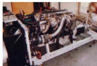
Carillo steel con rods giving an 8:1 compression ratio. All moving parts have been dynamically balanced, making for smoother running. To improve cooling further a larger diameter impeller was fitted to the water pump while more secure screw-in brass core plugs replaced the standard steel push-fit items. Drive belt pulleys were ditched in favour of lightweight aluminium versions.
