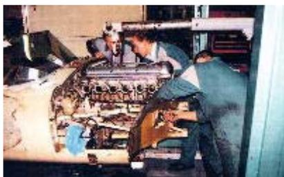
With trepidation and a feeling of great responsibility, Lynx's technicians began stripping the car to the tub. Bonnet and hard top were removed first, along with the seats. Engine and gearbox came next and as with all lightweights, the front picture frame has to be removed first. Front and rear suspension followed. Every stage was captured on film.
