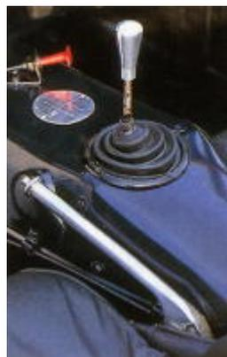
The gearbox is a ZF five-speed supplied by Jaguar as an option but never used. 'The gate is widely spaced so it's obvious which gear you are going into. It's very nicely sprung, especially third-to-fourth, and there is no vibration coming through the lever. The clutch, like the other controls, is smooth and easy to control and just a bit heavier than the road car's'.
