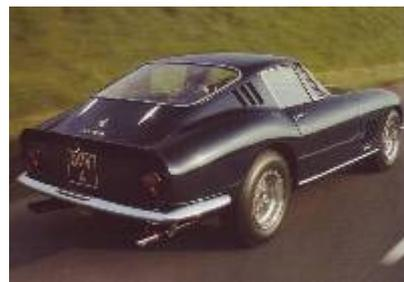
Although by no means as lusty as the Daytona, with just 3.3-litres, the 275GTB/4 motor is a big improvement in grunt over its predecessor, and it has enough torque to help you along until the gearbox oil has warmed through. Its 300bhp at 8000rpm and 202lb ft of torque at 5500rpm come on strong, and while this car weighs 152kg more than the 250, it is also a hefty 272kg lighter than the Daytona.
